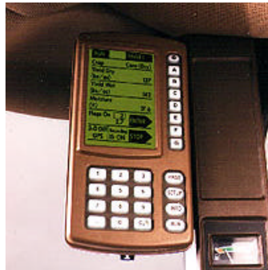
Figure 4 Operator's console mounted in the combine cab. (Courtesy of Deere and Co.)
